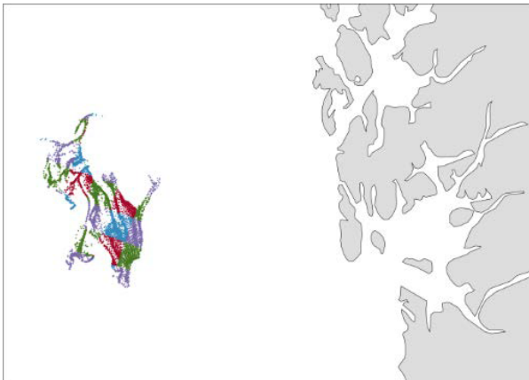
Figure 1 – Dividing particles among processes with a checkerboard scheme.
