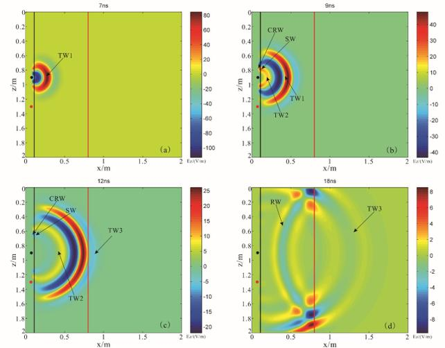
Figure 2 – Snapshots of the vertical component of the electric field in the simulation of water-base mud (The black dot represents the position of the transmitting antenna. The red dot represents the position of the receiving antenna, and the black solid line indicates the location of the borehole. The red solid line represents the interface between the invaded zone and the virgin formation).
