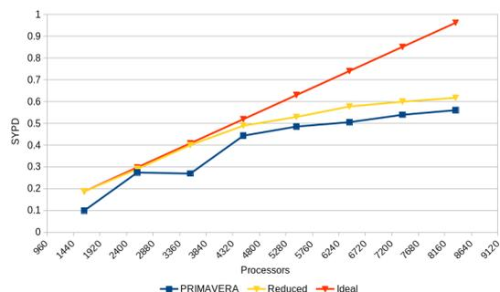
Figure 1 – Scalability test for the Glob-12km. Simulated Years Per Day as a function of the n. of cores used for two different set of outputs
