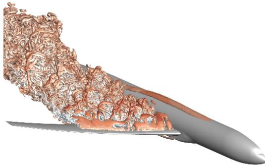
Figure 1 – Common Research Model wake at  $M_\infty = 0.25$ ,  $Re = 11.6 \cdot 10^6$ ,  $\alpha = 18^\circ$
