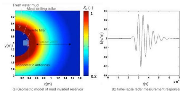
Figure 1 – The established mud invaded model with borehole radar (a) and the corresponding EM responses (b).
