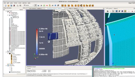
Figure 1 – SMITER GUI study running on compute node of tegner.pdc.htb.se showing in the centre window peak power deposition of 2.2 MW/m<sup>2</sup> on the target panel that is combined with the ITER blanket CAD geometry inside a ParaView window. Mesh detail of the target is shown in the right window.
