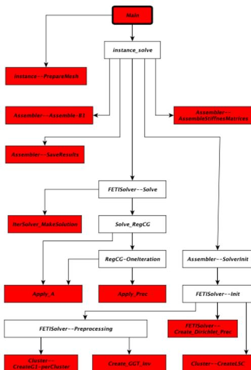
Figure 1 - Diagram of significant regions of the ESPRESO FEM library. The red regions are used for dynamic tuning.
