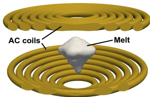
Figure 1 – Simulation of levitating liquid metal.
