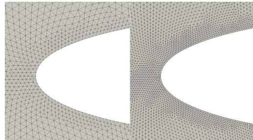
Figure 1 – Mesh multiplication algorithm applied to an airfoil (leading edge). Unrefined case, left; refined case, right.
