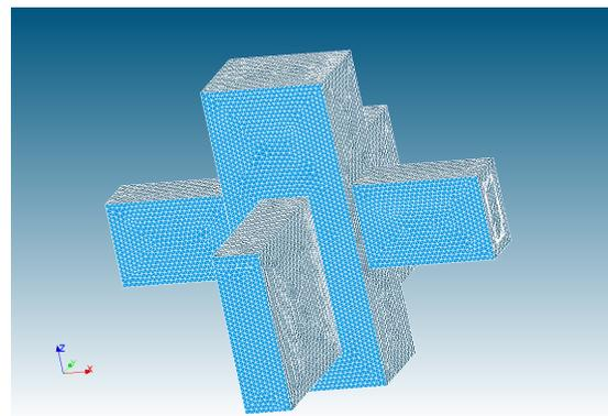
Figure 2 - Fine scale model for the main structural joint.
