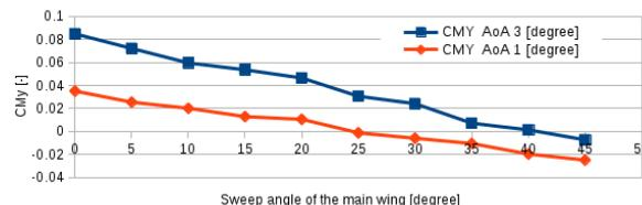
Figure 2 - Effect of variation of the sweep angle on the CM<sub>y</sub>
