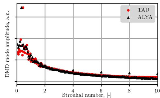
Figure 2 – CRM normalized dynamic mode spectrum at the wake plane at 28.3% of semispan
