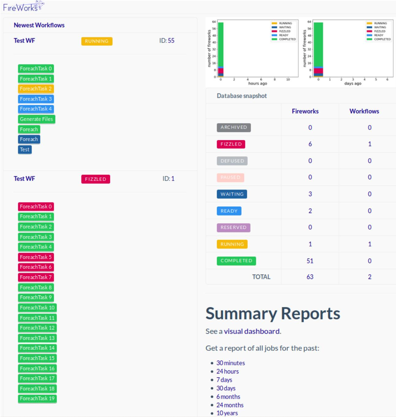
The screenshot displays the FireWorks web interface. On the left, two workflow cards are shown: 'Test WF' (ID: 55) in a 'RUNNING' state and 'Test WF' (ID: 1) in a 'FIZZLED' state. Each card lists its constituent tasks. The 'Test WF' (ID: 55) tasks are: ForeachTask 0, ForeachTask 1, ForeachTask 2, ForeachTask 3, ForeachTask 4, Generate Files, Foreach, Foreach, and Test. The 'Test WF' (ID: 1) tasks are: ForeachTask 0 through ForeachTask 19.
