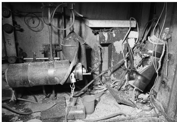
Figure 6. This also happened occasionally—consequences of an explosion in a small fume hood of the fluorine laboratory.
