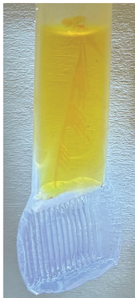
Figure 1. Needle-shaped crystals of [XeF][PtF 6 ]( mP108 ) growing from an aHF solution contained in an FEP tube (6 mm internal diameter; 8 mm outer diameter).
